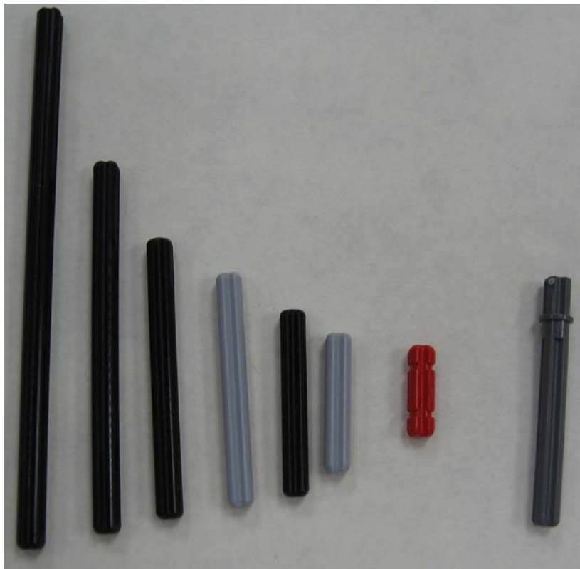
Figure 7. Cross-axles from the NXT kit.
